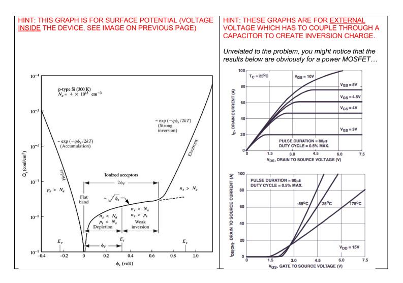
(2) Some multiple choice questions for NMOS. For the 1<sup>st</sup> few, remember that charge generation under the gate of a MOSFET follows either only depletion (dopant atoms) or Fermi-level shift type effects (carrier generation). Pick one answer for each. Do MORE than just look at the curves above, make sure you UNDERSTAND why as well!
